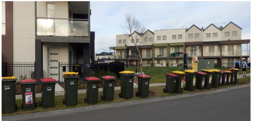
Allowance should be made for bins to be located such that there is a minimum 600mm (60cm) between each bin to aid in efficient collection by waste collection trucks. This will allow for the placement of both garbage and recycling bins, while also providing sufficient spacing for the waste collection contractor to pick up and put down bins without interfering with adjacent bins. Drivers of waste collection vehicles will not leave a vehicle to arrange or move bins.
