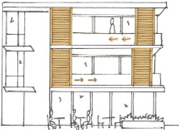
Figure 28: operable elements that provide shading and screening
