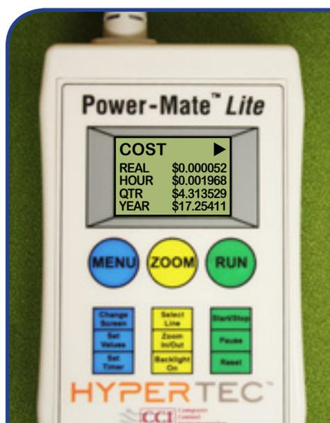
3. Find out the costs of your appliance by clicking the **Menu** button (a few times if needed) until you are in the Cost screen. This shows the real, hourly, quarterly and yearly cost (\$) to run the appliance. Real cost is the cost to run the appliance since the Power-Mate measurement started – this is useful to find out cost per use. Hourly, quarterly and yearly costs are based on constant usage of the appliance over that time period.
