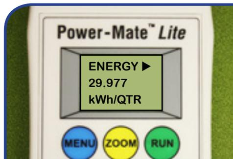
2. Click the **Run** button to start the measurement. A flashing ► will appear in the top right corner of the screen to show that the Power-Mate is measuring the energy use of the appliance.
