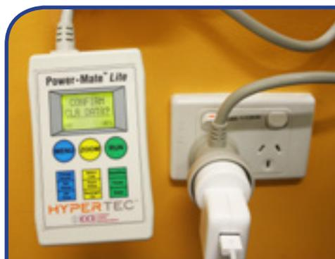
1. Plug in the Power-Mate to a power point and plug your appliance into the Power-Mate socket.
