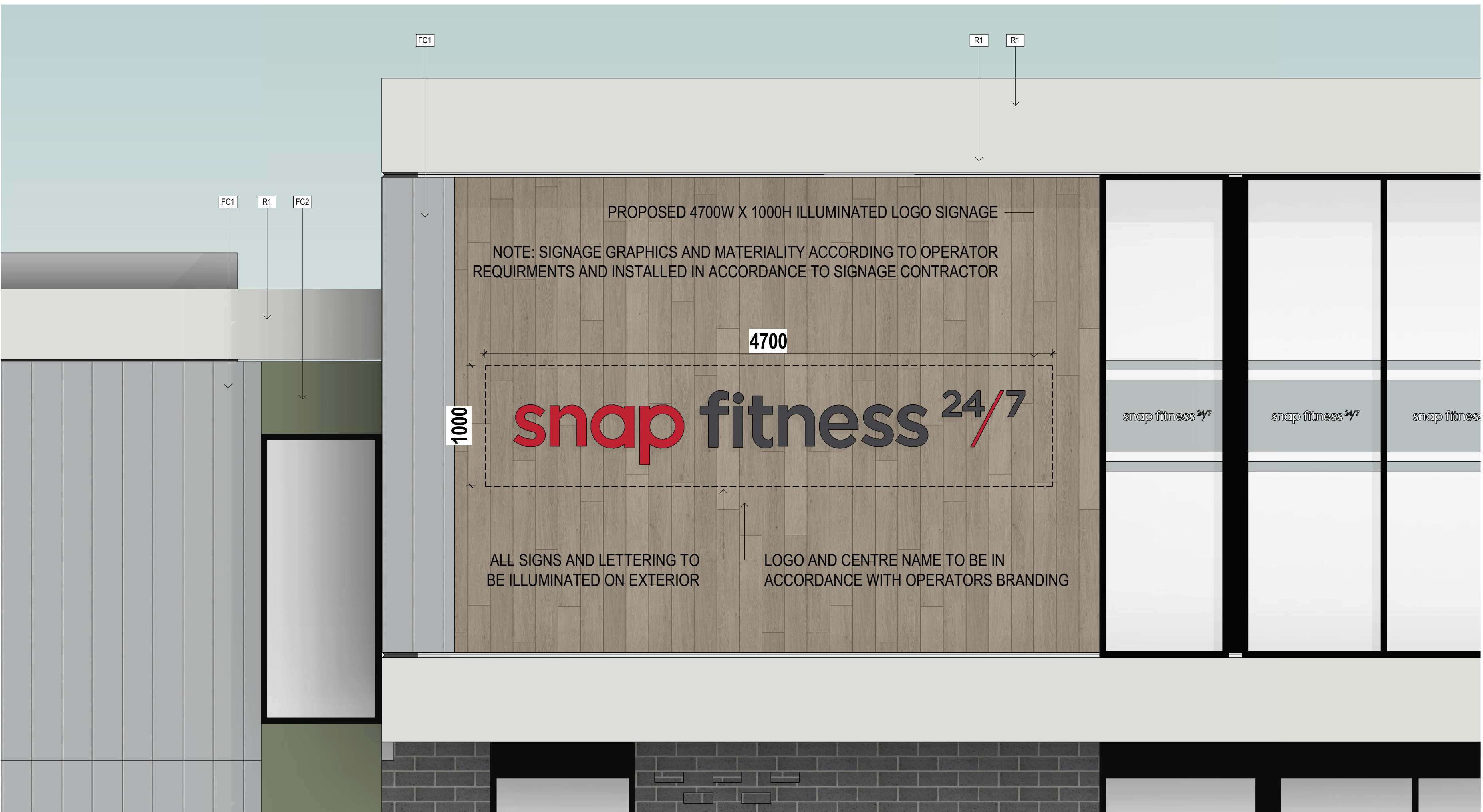
2 TYPICAL SIGNAGE ELEVATION - FITNESS CENTRE TP400 SCALE 1 : 25
