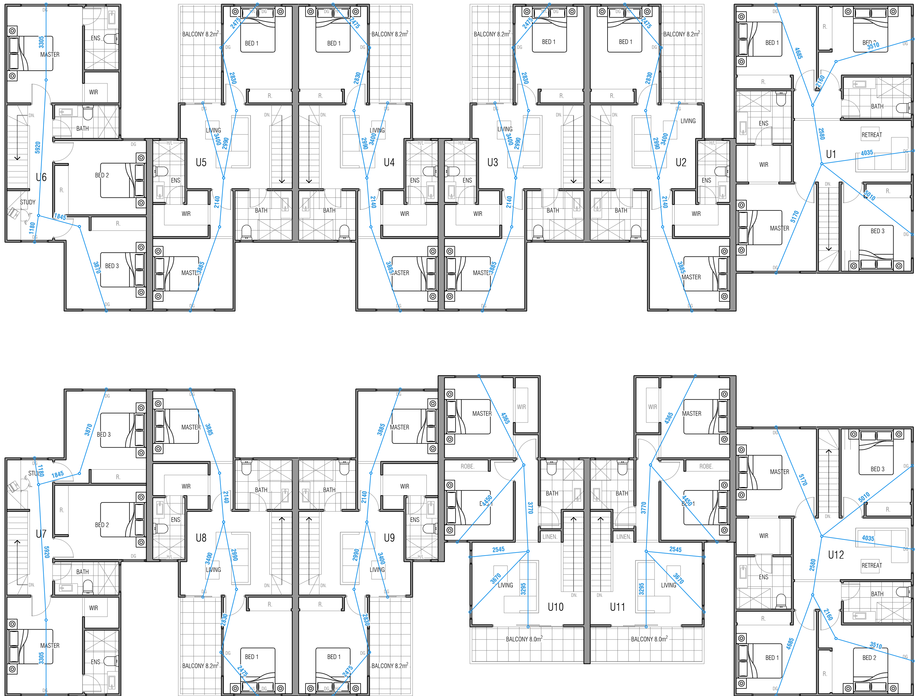
FIRST FLOOR PLAN CROSS-FLOW VENTILATION DIAGRAMS SCALE 1:100
