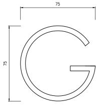
THIS SYMBOL SHALL BE STAMPED INTO THE FACE OF THE KERB IMMEDIATELY ABOVE THE POSITION WHERE A GAS SERVICE CONDUIT IS PLACED ACROSS THE ROADWAY.
