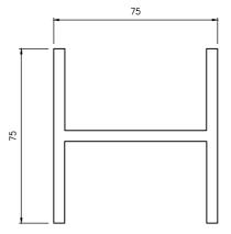
THIS SYMBOL SHALL BE STAMPED INTO THE FACE OF THE KERB IN LINE WITH THE POSITION WHERE A PROPERTY STORMWATER CONNECTION IS PROVIDED TO AN UNDERGROUND STORMWATER PIPE OR PIT.
