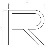
THIS SYMBOL SHALL BE STAMPED INTO THE FACE OF THE KERB IMMEDIATELY ABOVE THE POSITION WHERE A RECYCLED WATER SERVICE CONDUIT IS PLACED ACROSS THE ROADWAY.
