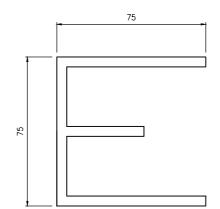
THIS SYMBOL SHALL BE STAMPED INTO THE FACE OF THE KERB IMMEDIATELY ABOVE THE POSITION WHERE AN ELECTRICAL SERVICE CONDUIT IS PLACED ACROSS THE ROADWAY.
