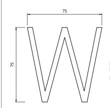
THIS SYMBOL SHALL BE STAMPED INTO THE FACE OF THE KERB IMMEDIATELY ABOVE THE POSITION WHERE A WATER SERVICE CONDUIT IS PLACED ACROSS THE ROADWAY.
