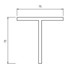
THIS SYMBOL SHALL BE STAMPED INTO THE FACE OF THE KERB IMMEDIATELY ABOVE THE POSITION WHERE A TELECOMMUNICATIONS SERVICE CONDUIT IS PLACED ACROSS THE ROADWAY.
