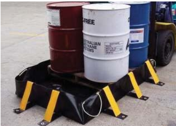
Bunding and kerbing
